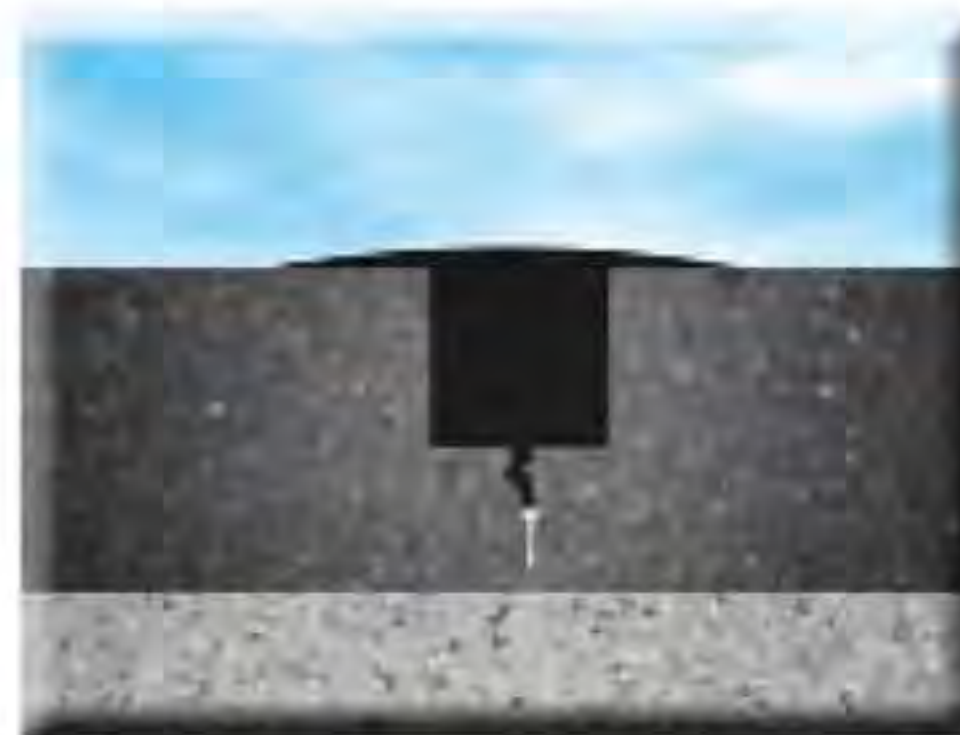
2. Standard Routed Crack
